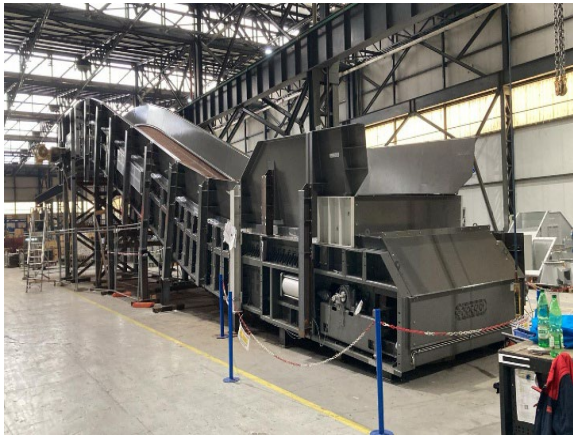
Assembly of Shredded Scrap Conveyor at Magaldi.
