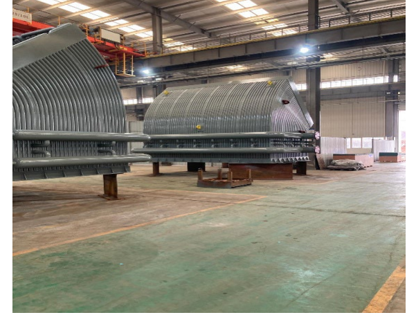
Consteel Offtaking and Settling Chamber
